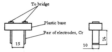
Fig. 1. Experimental probe sensor for measurements in whole apples.
