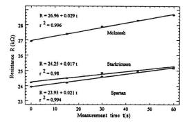
Fig. 3. Apple electrical resistance versus measurement time in commercial harvest date.
